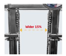
Adopt the new-type of box iron. Increase the inside width of inner mast and the spacing between lifting cylinders. The lowering of instruments in the cabin will greatly increase the forward visibility; The rear visibility will also be greatly improved through the optimization design of counterweight.
