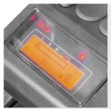
Newly-developed LCD instrument has more comprehensive functions and more stable performance and entirely displays the full truck state, fault code and other important information, which can make the operator more intuitively and conveniently have a better knowledge of truck state and make the maintenance conveniently.
