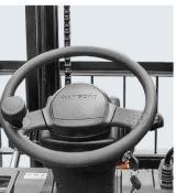
The design of steering wheel of small diameter and electro-hydraulic reversing as well as the car-type double-handle combination switch will greatly improve the driving comfort.
